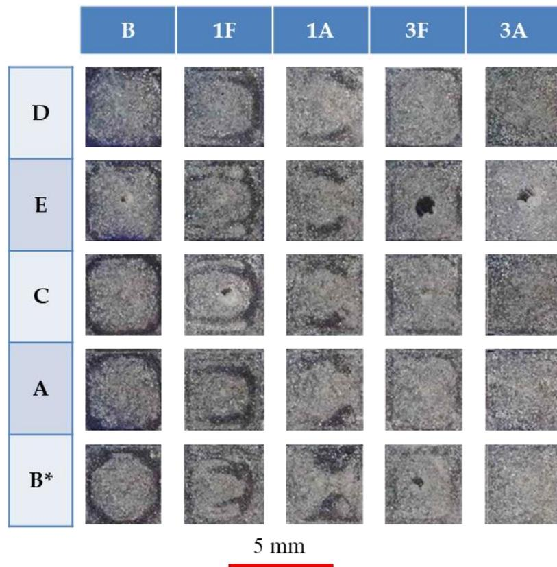
**Figure 2.** The microscopic images created from the cross-sections of different regions with different injection moulding settings.
